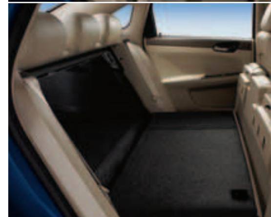
The innovative flip-and-fold-flat rear seats create an extended loading floor that is 1905 mm (75 in.) in length – more than long enough for oversized items, such as skis.
